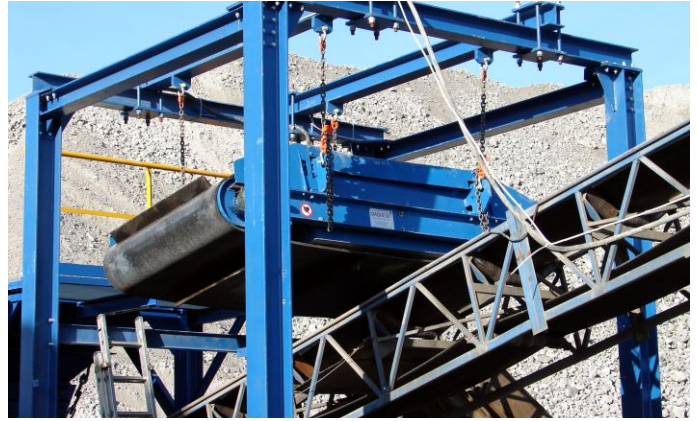
Ferrous scrap recovery from metallurgical slag.
