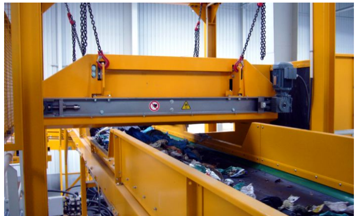
Ferrous scrap recovery from municipal waste.
