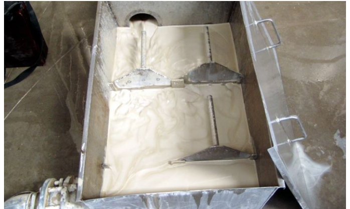
Tub filter for removal of iron contaminants from liquid ceramic body.
