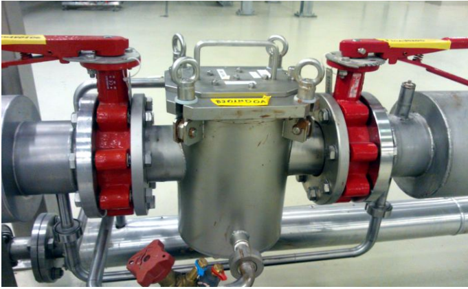
Filter installed horizontally for removal of fine iron contaminants from liquid chocolate.
