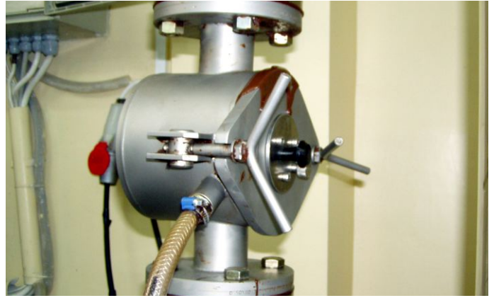
Filter installed vertically for removal of fine iron contaminants from liquid chocolate.
