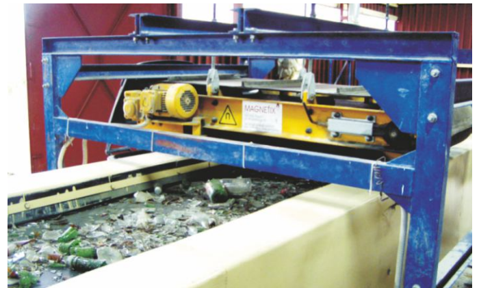
Separation of ferrous scrap from glass cullet.
