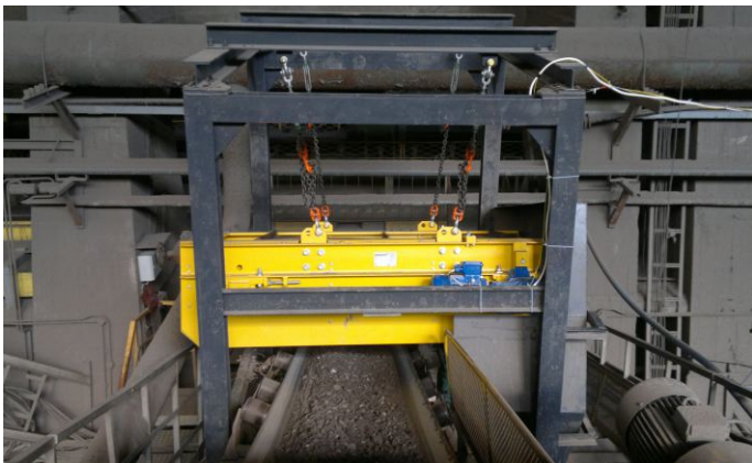
Removal of tramp iron contaminants from copper ore.
